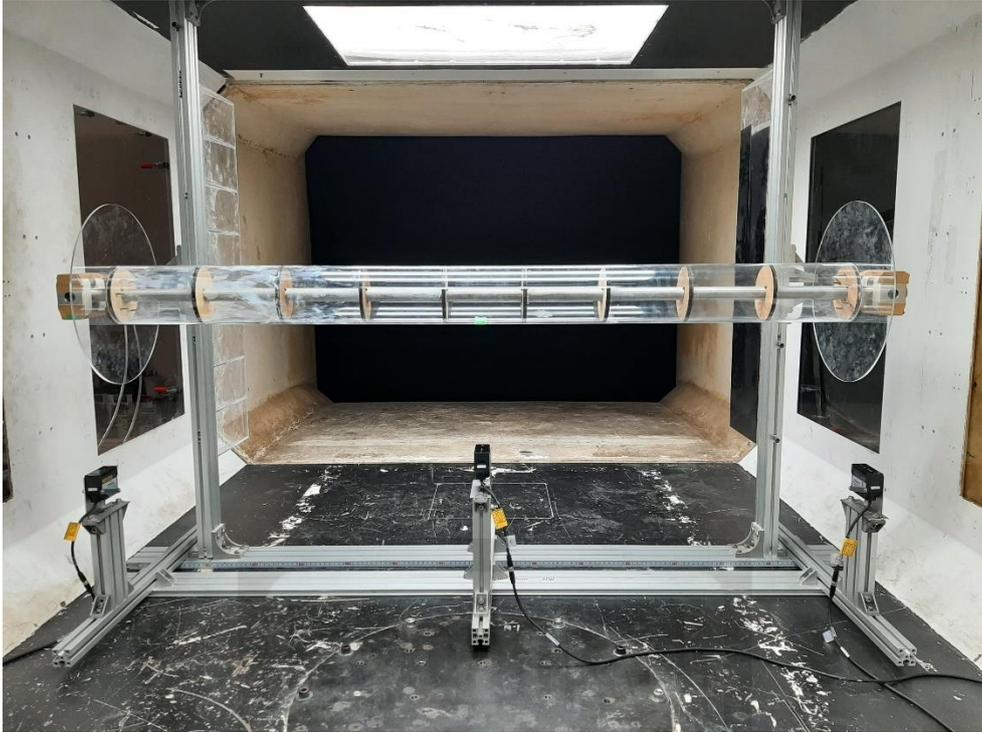
Figure 3.3. Cylinder (Model 2) used for vibrating tests installed in the low-speed wind tunnel. Three laser sensors were used to measure the amplitude of vibration.
