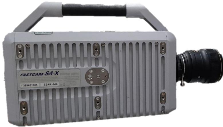
Figure 3.5. High speed camera Photron Fastcam SA-X.
