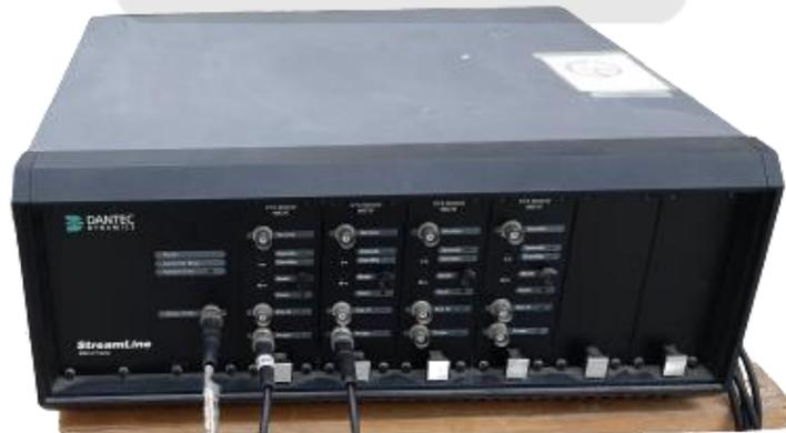
Figure 3.10. DANTEC Streamline Pro CTA 90C10 system.
