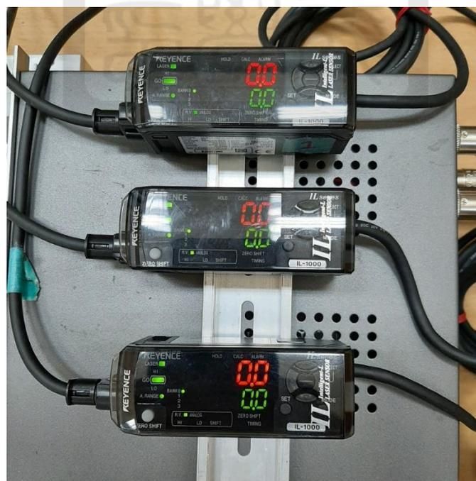
Figure 3.20. The laser sensors KEYENCE IL-1000.
