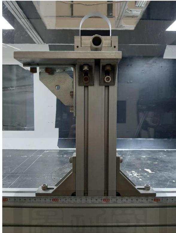
Figure 3.23. Structure that supports the model for the static experiments.
