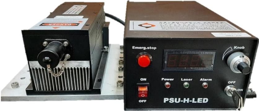
Figure 3.4. Green laser DPSS 532 nm – 5W.
