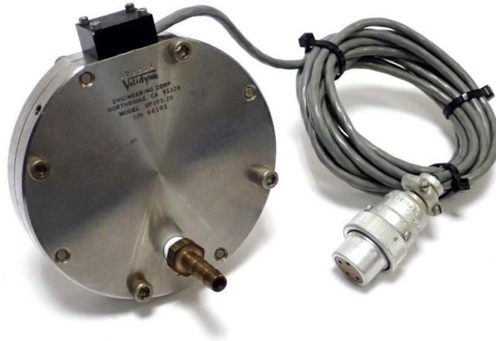
Figure 3.15. Validyne DP103-18 low pressure variable reluctance sensor.
