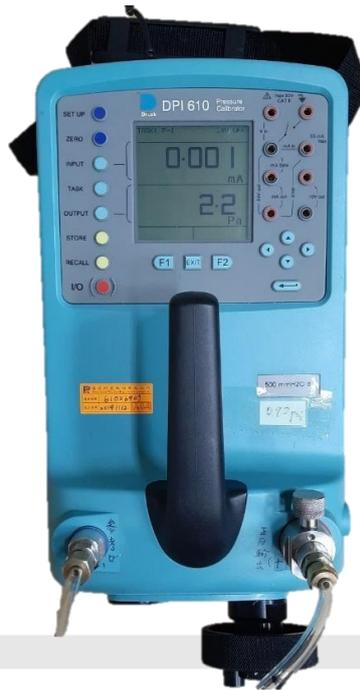
Figure 3.13. Low pressure calibrator DPI610.
