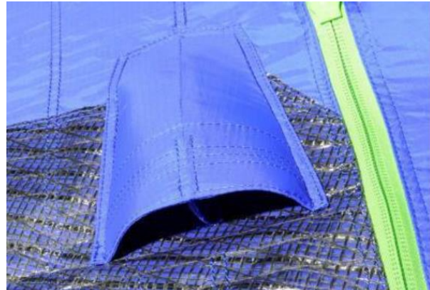
Figure 2. A close-up of a reinforced wingsuit ram-air inlet.
