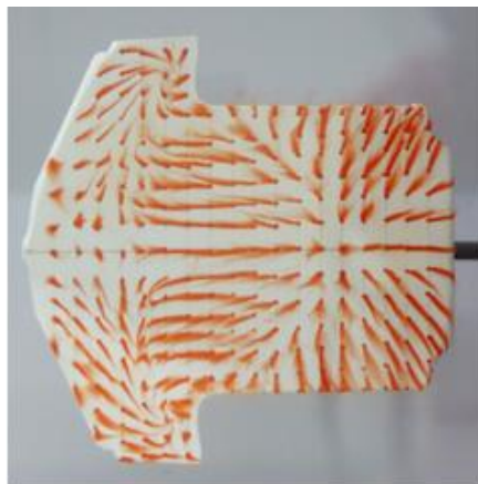
Figure 35. AURA arms 1 (left) and arms 2 (right) models during red dot method test at different AOA.
